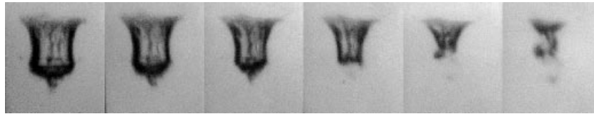
FIGURE 10. Jet-like ejection of boundary material during bubble collapse near an elastic boundary, \gamma = 0.1 . The photographic sequence is taken by using diffuse illumination with 10^6 frames s^{-1} (frame interval 1 \mu s ). Frame width 1.4 mm.
